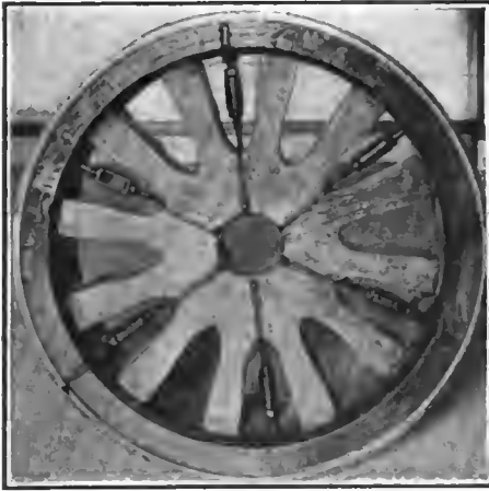
New Turner patent wheel for heavy duty, by means of adjustable wedges it is possible to tighten up the wheel on the road
